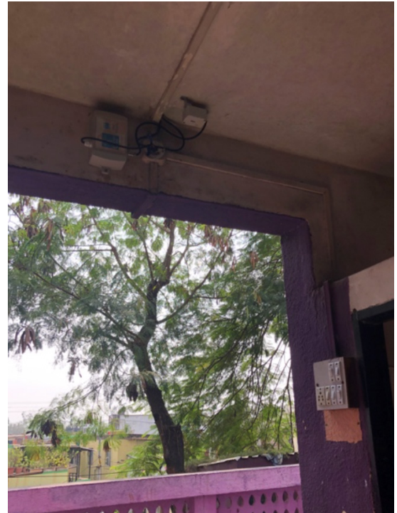
At the top of the doorway is one of Samagra's sensors that measures foot traffic
